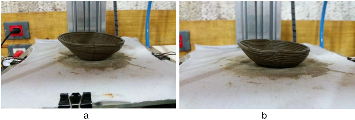
Figure 5 - Collapsed specimens. (a) slope of 51°; (b) slope of 52°
